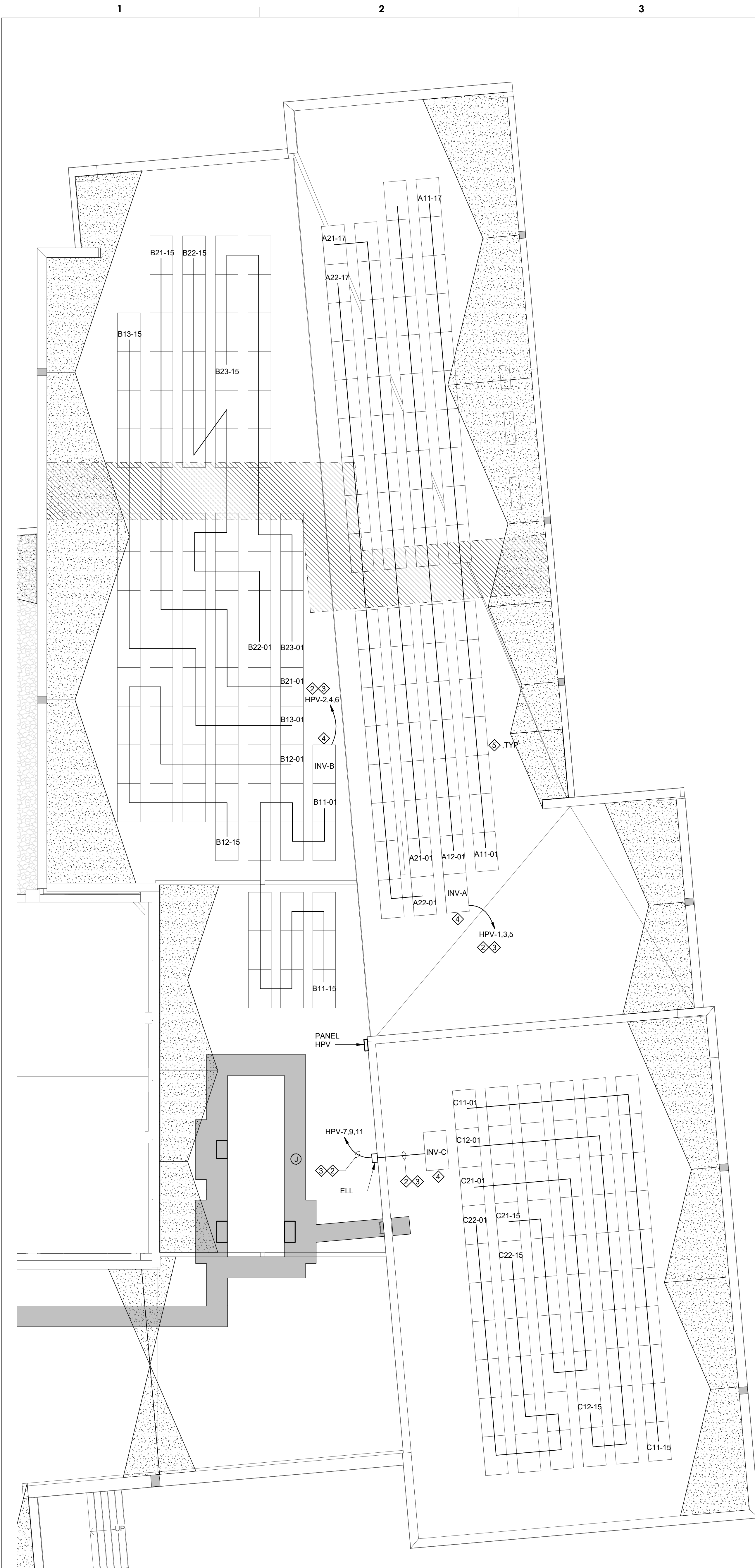
2 PHOTOVOLTAIC STRING LAYOUT 1 E3.6 1/8" = 1'-0"
